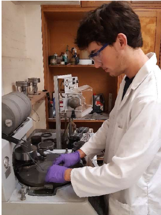
Figure 5: Author using the Logitech LP50 lapping machine in the preparation of samples for bonding with slides.
