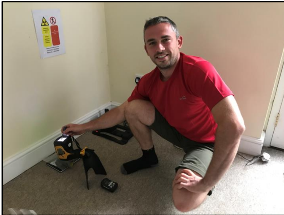
Figure 14 (left): The SHG Olympus Delta Premium Alloy Plus Analyser (DP2000) being calibrated by Geologist Jamie Price. Prior to sample analysis, the pXRF device was calibrated by scanning 3 samples of known composition that were created by SHG. The pXRF was set to soil mode which ran two 30kv beams each lasting 15 seconds. (photo taken by author on 09/07/21)
