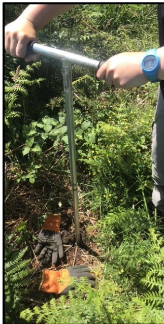
Figure 12: Auger being used in the field, with an annotated soil sample to highlight different soil horizons seen in the field (photos taken by author on 13/08/21)
