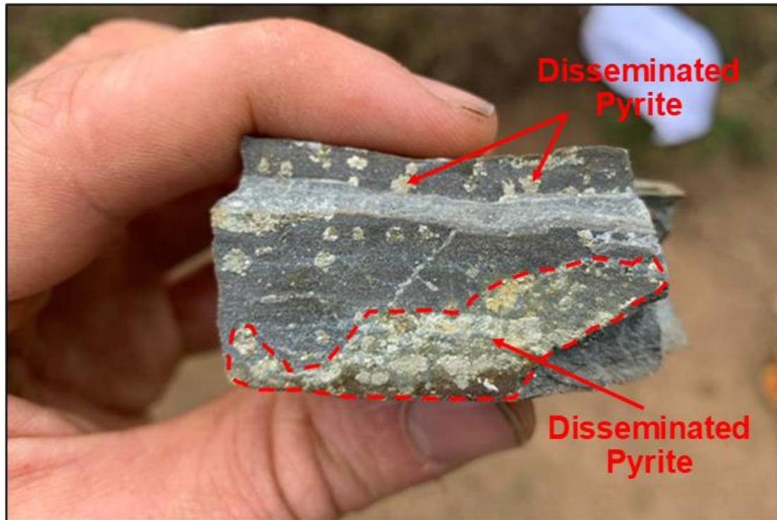
Figure 13: Photo of a rock chip sample collected at an outcrop of the Nant-y-Coy Formation. The sample is a laminated, siliceous siltstone with abundant disseminated pyrite. Thumbnail is 1cm for scale. (photo taken by author on 27/07/21)
