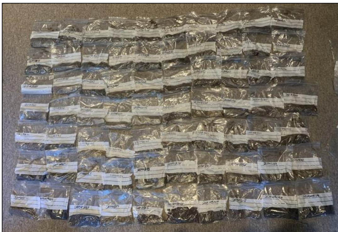
Figure 10: Soil samples laid out for appropriate QAQC procedure involving photography, weighing of samples, digitizing paper data sheets onto Microsoft Excel and uploading GPS tracks (photo taken by author on 13/07/21)
