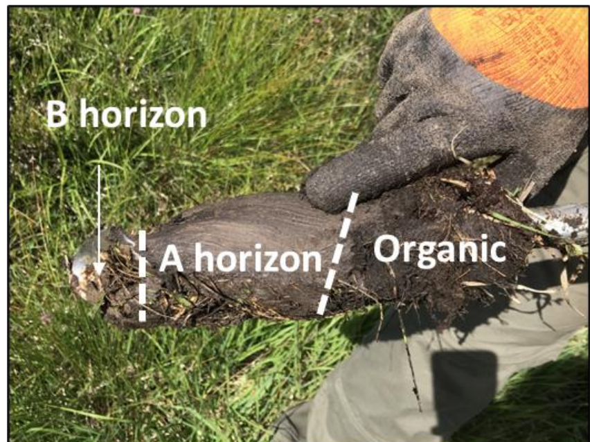
Figure 12: Auger being used in the field, with an annotated soil sample to highlight different soil horizons seen in the field (photos taken by author on 13/08/21)
