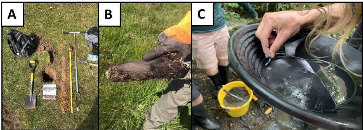
Figure 5: a) Photograph showing the required equipment needed for soil sampling, including an auger, shovel and sample bag b) Soil sample extracted via the auger c) Geologist extracting gold grains from panned concentrate (photos taken by author from 12/08/21 to 13/08/21)
